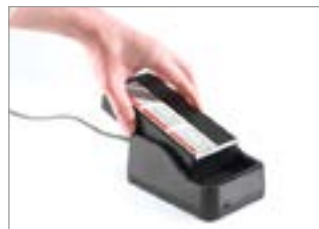
21 - Docking station for removable battery
